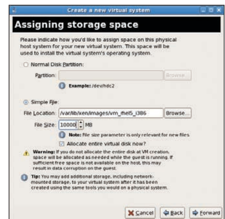
Figure 3. “Assigning storage space” step when creating a virtual machine in Red Hat Enterprise Linux 5 Virtual Machine Manager
